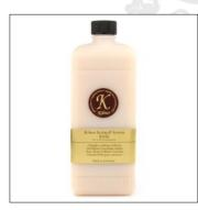
Like most other water-based products, Instacoll is best applied at moderate temperatures. The optimum temperature for application is between 15 and 25°C. Between 5 and 15°C the product must be thinned more to ensure the correct consistency and flow is maintained. At temperatures below 5°C the product cannot be used and at temperatures above 25°C only small areas can be gilded.
