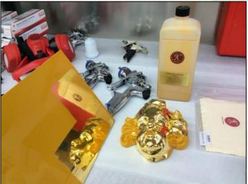
you should always use professional-quality equipment. The manufacturer of the Instacoll System tested with SATA brand spray equipment and achieved good results. Any other similar high-end brand should would just as well. The main factor in the quality of the finish is the accuracy and skill of the craftsperson applying it.
