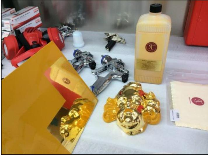
manufacturer of the Instacoll System tested with SATA brand spray equipment and achieved good results. Any other similar high-end brand should would just as well. The main factor in the quality of the finish is the accuracy and skill of the craftsperson applying it.
