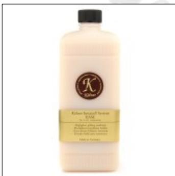
Like most other water-based products, Instacoll is best applied at moderate temperatures. The optimum temperature for application is between 15 and 25°C. Between 5 and 15°C the product must be thinned more to ensure the correct consistency and flow is maintained. At temperatures below 5°C the product cannot be used and at temperatures above 25°C only small areas can be gilded.
